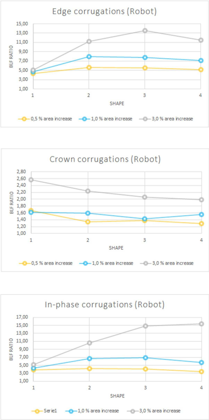
Figure 4.3.4 – The buckling load factor for edge-, crown- and in-phase corrugations of a barrel vault using Autodesk Robot
